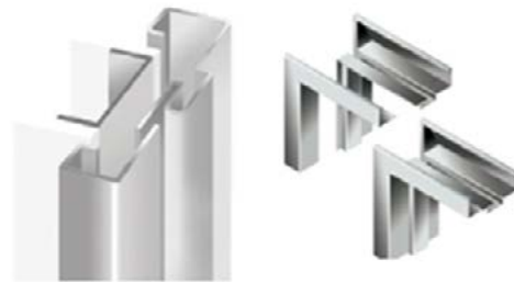
Split frame wrapping steel stud with drywall.
