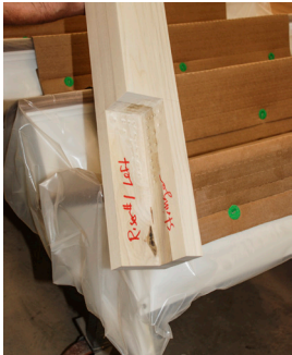
Post is notched for exact location and height.
